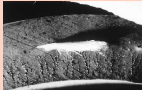
Tube cracking due to electrochemical degradation.
